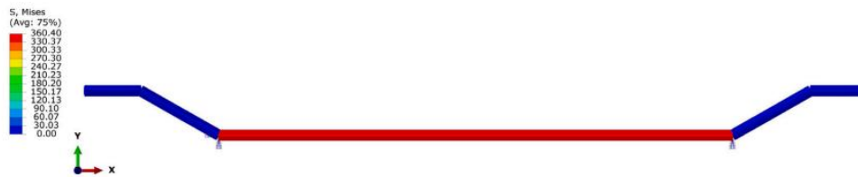
Fig. 19. Recovery stress distribution in the Fe-SMA fiber under activation, with encastre boundary conditions applied at supports (in MPa).
