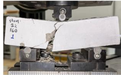
Fig. 4. The test procedure and setup for three-point bending at (a) Phase I, and (b) Phase II loading.
