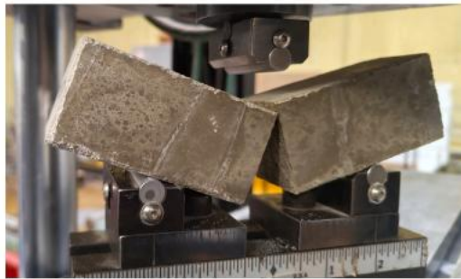
Fig. 5. Determination of (a) flexural and (b) compressive strength of concrete based on EN 1015-11.
