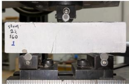
Fig. 4. The test procedure and setup for three-point bending at (a) Phase I, and (b) Phase II loading.
