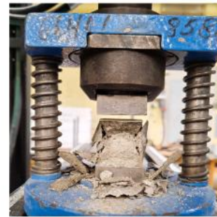
Fig. 5. Determination of (a) flexural and (b) compressive strength of concrete based on EN 1015-11.
